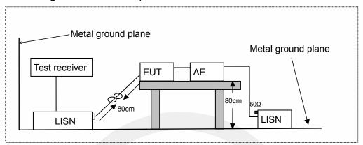
LISN: Line Impedance Stabilization Network
