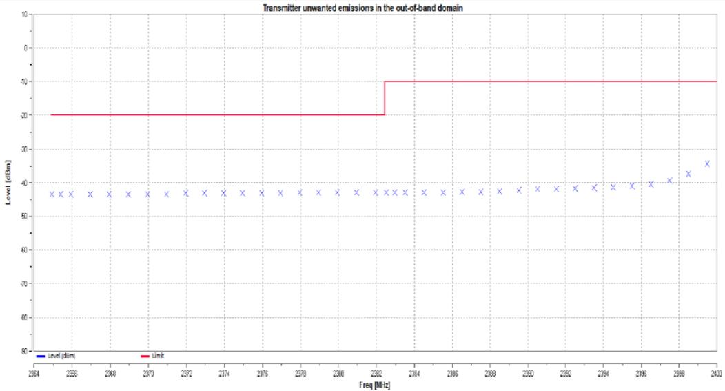
**Transmitter Unwanted Emission In The Out-Of Band**
