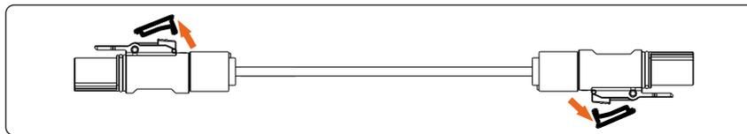
3) Push the plastic button on each end of the power cable in the direction of the arrow
