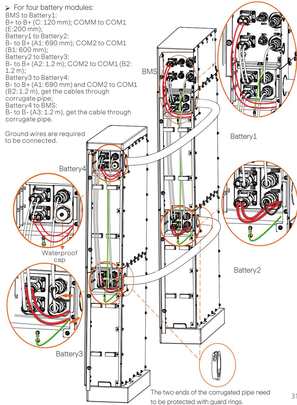
The two ends of the corrugated pipe need to be protected with guard rings.
