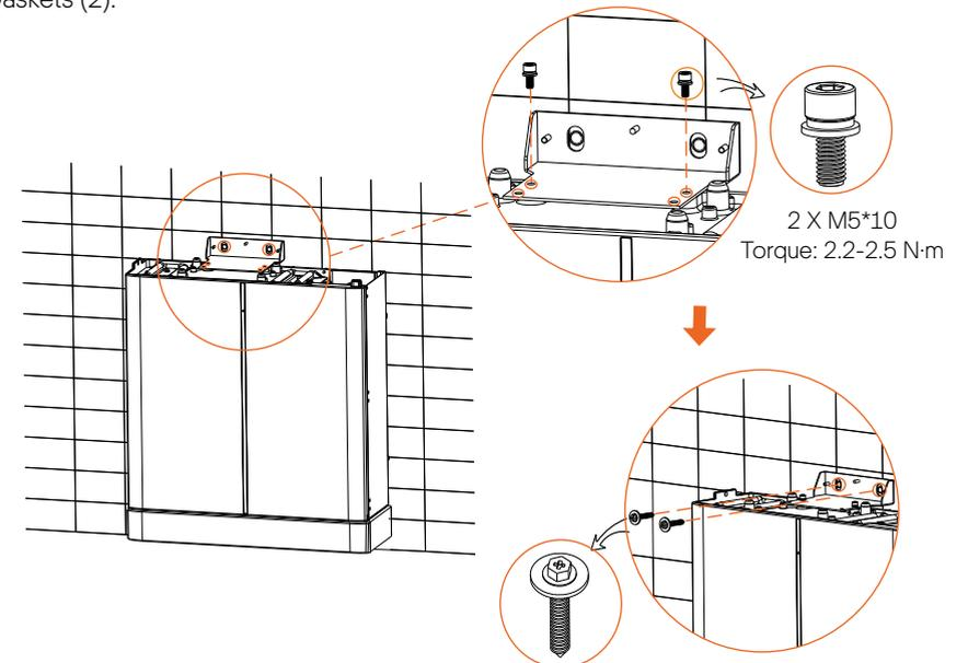
Step 6: Place BMS on the top of the battery module, and secure both left and right sides with M4 screws (2). See figure below.
