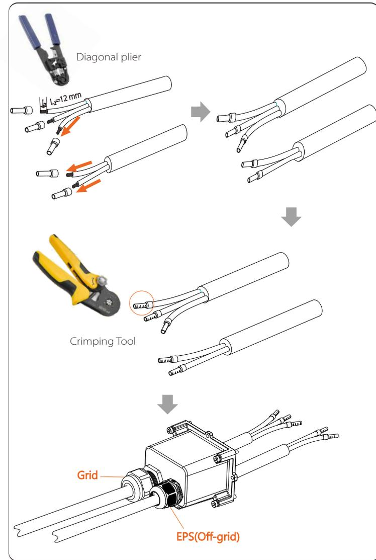
**Step 4.** Find the location of the AC interface on the inverter, insert the crimped terminals into the UW10 terminals L, N, and P according to the wire sequence, and use a flat-blade screwdriver to tighten the screws. (Torque:  $1.5 \pm 0.1 \text{ N} \cdot \text{m}$ )
