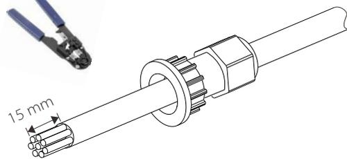
**Step 3.** Insert the prepared communication cables into the RJ45 terminals in sequence, and then use network cable crimping pliers to press them tightly.
