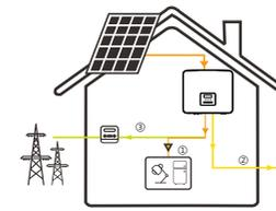
The back-up mode is suitable for areas with frequent power outages. This mode will maintain the battery capacity at a relatively high level, to ensure that the emergency loads can be used when the grid is off. Same working logic with "Self-use" mode.
