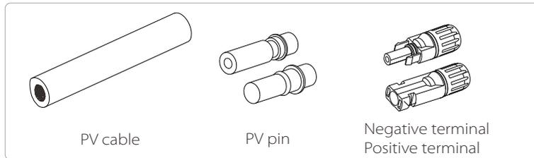
**Step 2.** Use a wire stripper to strip the 7 mm insulation layer of the wire end.
