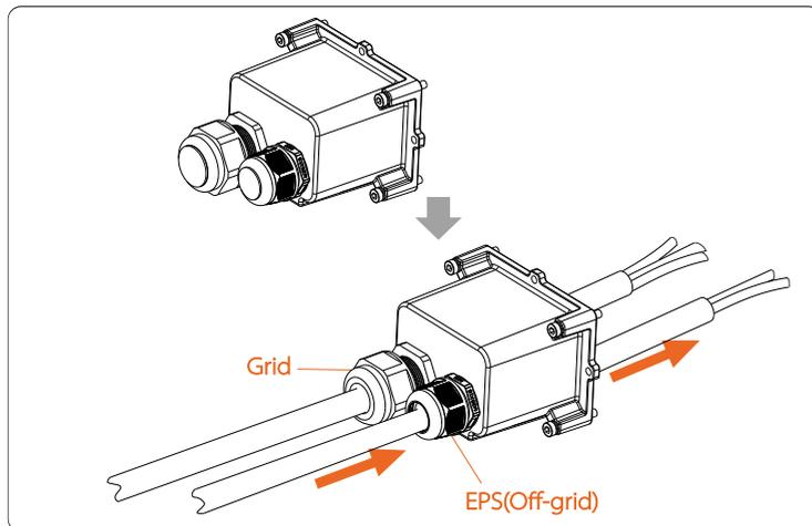
**Step 3.** Remove the 12 mm insulation layer at the end of the wire. Insert the European-style terminals respectively, and make sure that the stripped ends are inserted into the European-style terminal, and finally use crimping pliers to press tightly.
