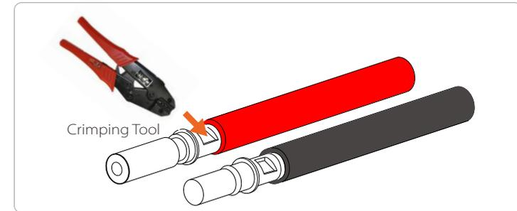
**Step 5.** The PV joint is divided into 2 parts - the plug and the fastening head. Insert the cable through the fastening head and the opposite plug. Notice that the red and black lines correspond to different of plugs. Finally, force the cable pair into the plug, will a "click" sound, which indicates that the connection is completed.
