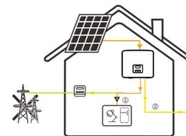
In case of power failure, the system will supply EPS loads through PV and battery.
