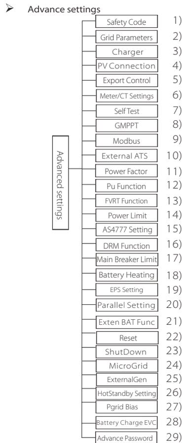
All advanced settings can be set here, such as battery, grid, EPS(Off-grid), etc.. "Advanced" setting is generally customization and resetting for battery and grid. Each part has lower level parts. Please contact your installer or factory and enter the installer password.
