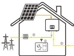
The back-up mode is suitable for areas with frequent power outages. This mode will maintain the battery capacity at a relatively high level, to ensure that the emergency loads can be used when the grid is off.
