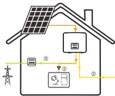
The self-use mode is suitable for areas with low feed-in subsidies and high electricity prices. The power of PV will supply the loads first, and surplus power will charge the battery, then the remaining power will feed into the grid.
