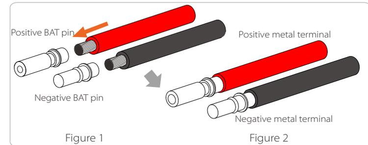
**Step 4.** Tighten the BAT pin contact and the wiring harness to make the connection tight without looseness
