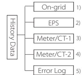
The history data contains five pieces of information: on-grid power of the inverter, EPS power generation, power of the meter/CT and error logs.
