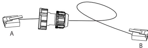
2) One side of the finished cable, Waterproof connector with RJ45 is inserted into the inverter, and one side of the RJ45 terminal is inserted into the CT connection.
