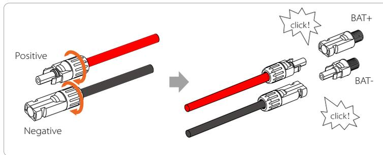
**Step 7.** Insert the battery power lines into the corresponding BAT port (+), (-) of the inverter.
