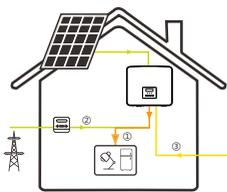
The feed-in priority mode is suitable for areas with high feed-in subsidies, but has feed-in power limitation. The power of PV will supply the loads first, and surplus power will feed into the grid, then the remaining power will charge the battery.
