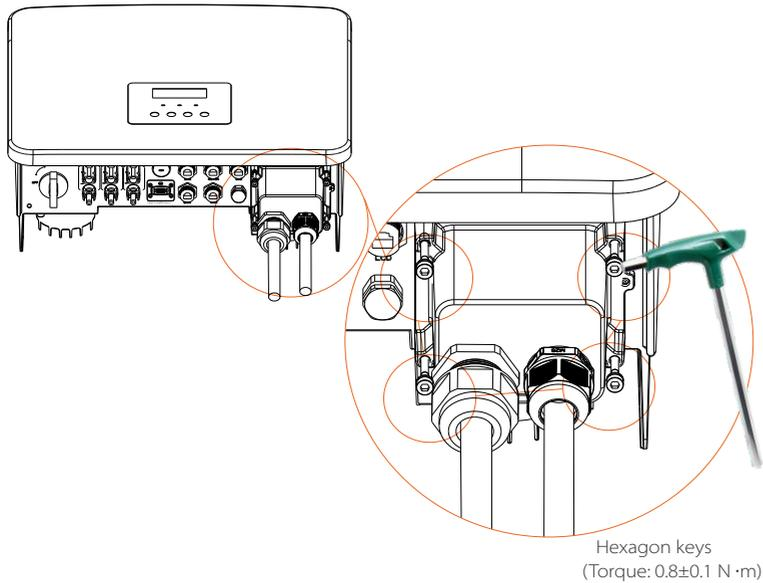
**Step 6.** Tighten the waterproof fastening head.
