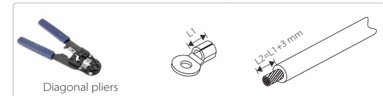
**Step 3.** Insert the stripped cable into OT terminal and tighten the terminal with a terminal crimping tool.
