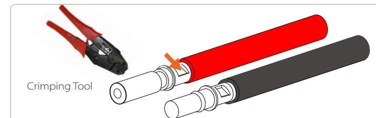
**Step 5.** The BAT joint is divided into 2 parts - the plug and the fastening head. Insert the cable through the fastening head and the opposite plug. Notice that the red and black lines correspond to different of plugs. Finally, force the cable pair into the plug, will a "click" sound, which indicates that the connection is completed.
